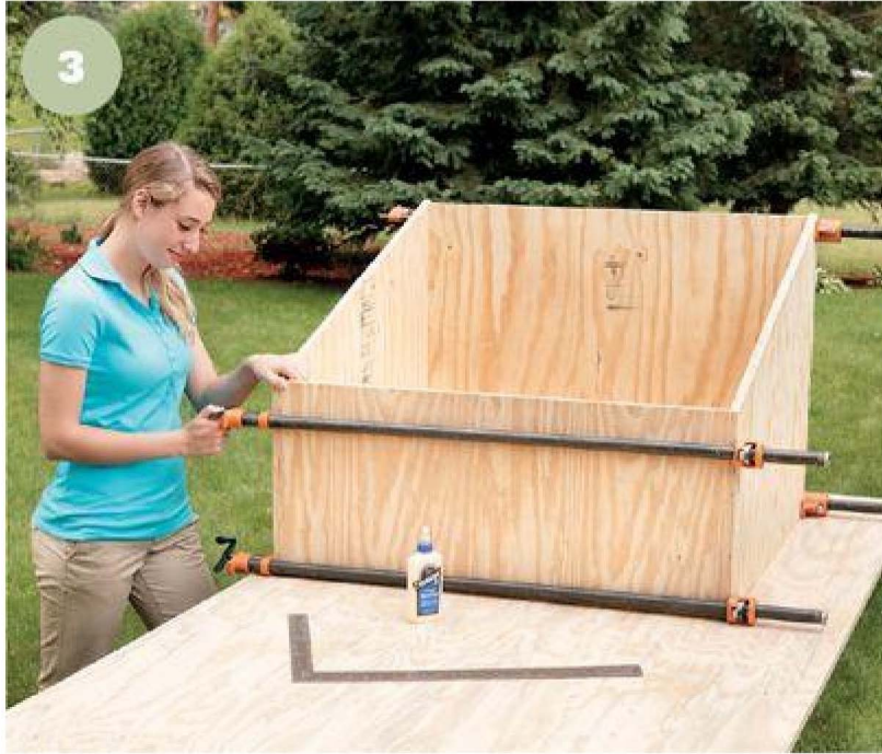
3 Assemble the front, back, and side panels into a square box. Glue the joints and clamp them together with pipe or bar clamps. Adjust until the corners are square.
