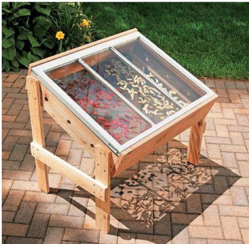
An old glass window sash gets new life as the heat-trapping cover of this solar dryer.
